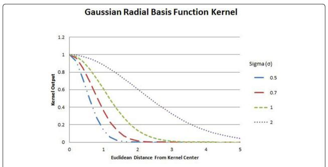
**Figure 6** Gaussian RBF kernel. The outputs of the Gaussian radial basis function kernel as functions of the Euclidean distance between vectors. Four functions are depicted in dashed-double-dotted-blue, long-dashed-red, dashed-green, and dotted-purple curves, corresponding to the cases where the sigma is 0.5, 0.7, 1.0, and 2.0 respectively.
