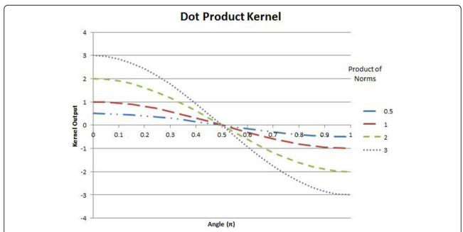
**Figure 4 Dot product kernel**. The outputs of dot product kernel as functions of the angles between vectors. Four functions are depicted in solid-blue, long-dashed-red, short-dashed-green and dotted-purple curves, corresponding to the cases where the product of the norms of the  $\vec{u}$  and  $\vec{v}$  vectors is equal to 0.5, 1, 2 and 3 respectively.
