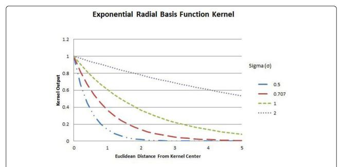
**Figure 7 Exponential RBF kernel**. The outputs of the exponential radial basis function kernel as functions of the Euclidean distance between vectors. Four functions are depicted in dashed-double-dotted-blue, long-dashed-red, dashed-green, and dotted-purple curves, corresponding to the cases where the sigma is 0.5, 0.707, 1.0, and 2.0 respectively.
