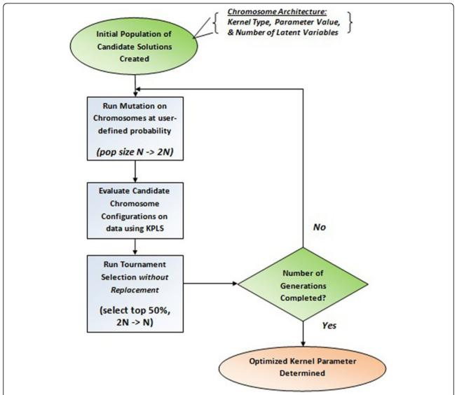
**Figure 3 Evolutionary Programming**. Shown is the process of the Evolutionary Programming optimization technique utilized to find the optimal kernel parameters. The process creates an initial population of candidate solutions (chromosomes) which undergo a stochastic search for the optimal parameter through the sub-processes of mutation and tournament selection of the 'most-fit' genes.
