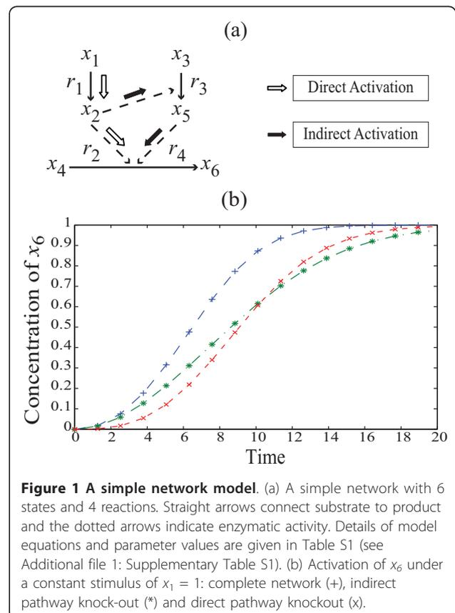
**Figure 1 A simple network model.** (a) A simple network with 6 states and 4 reactions. Straight arrows connect substrate to product and the dotted arrows indicate enzymatic activity. Details of model equations and parameter values are given in Table S1 (see Additional file 1: Supplementary Table S1). (b) Activation of  $x_6$  under a constant stimulus of  $x_1 = 1$ : complete network (+), indirect pathway knock-out (\*) and direct pathway knockout (x).
