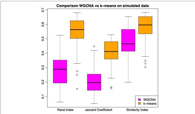
**Fig. 4** Results on performance of standard WGCNA and k-means on 42 simulated data sets that used the GTEx WGCNA GNCs as seed for simulation. We display the same results using three different indexes of similarity between cluster partitions. The k-means method outperforms standard WGCNA with all three indexes used
