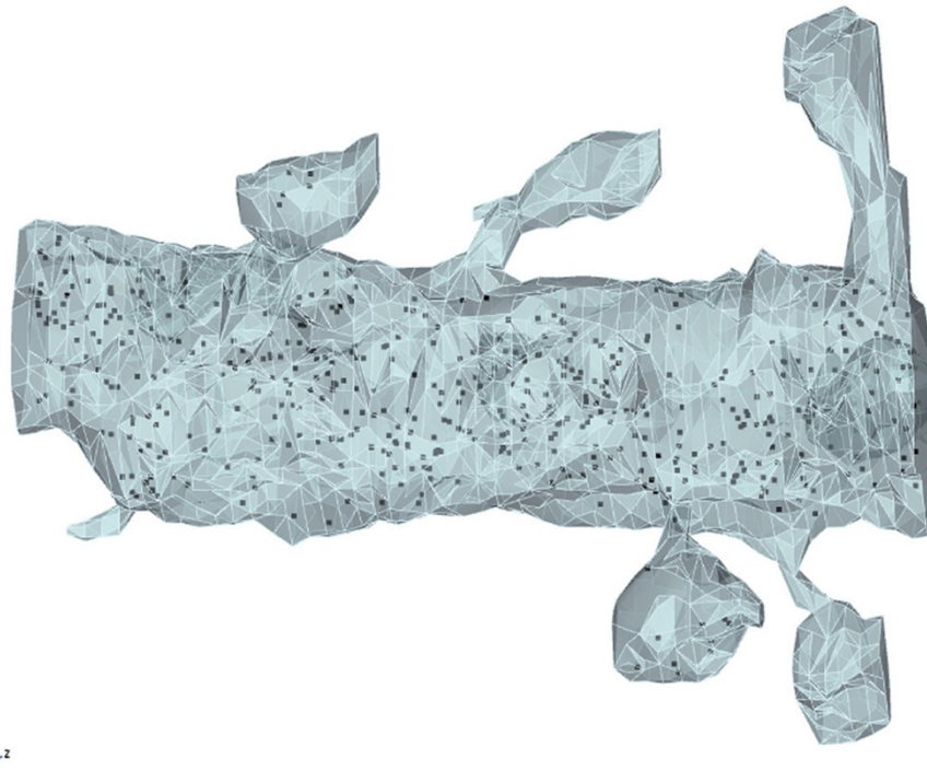
Figure 2 STEPS import of a tetrahedral mesh with realistic geometry. The mesh is reconstructed from a surface triangular mesh provided at http://synapses.clm.utexas.edu/anatomy/Ca1pyrmd/radiatum/K24/K24.stm . For a test simulation in STEPS molecules are distributed uniformly and the system is then visualized in CUBIT.
